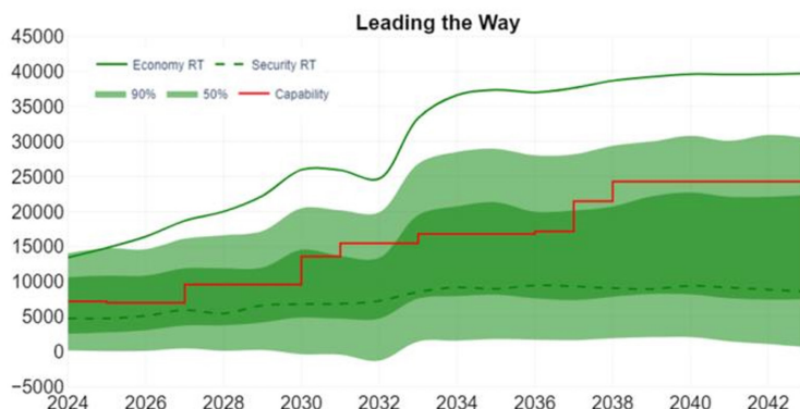
Figure 9: Illustration of planned transmission capability between Scotland and England (red line) and the distribution of required transfers under the Leading the Way scenario. Based on transmission projects which have currently been given the go ahead by Ofgem, transfer capability is expected to grow to around 16 GW by the mid 2030s 59 .
